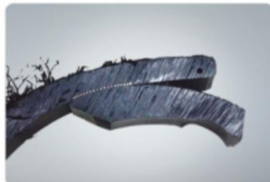
Peel Testing Specimen
