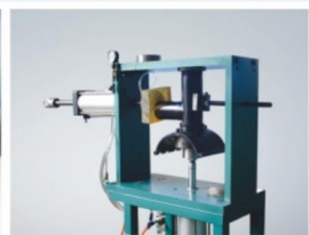
Tapping Saddle Impact Resistance Testing Equipment
